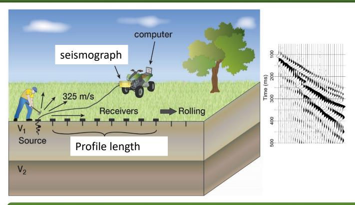
Illustration of the MASW Method in the surveying
