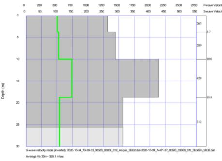
Inverted 1-D Velocity layer model of the selected stations
